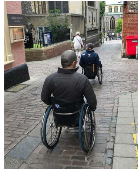
14 - Uneven surface Incline 1:7 along St Andrews Hill
