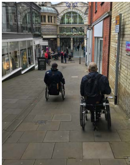
13 - Incline 1:7 along Arcade Street
